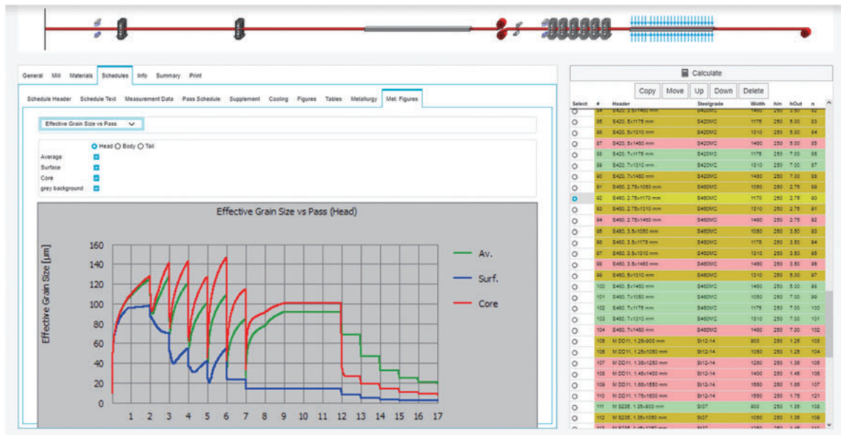
図6：Grain size evolution indicating normal rolling part (roughing rolling steps 2-7) and thermomechanical rolling during finishing passes (steps 12-17).
