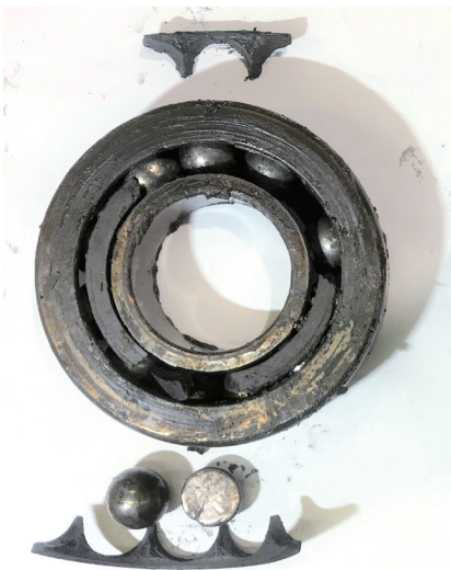
Damaged Bearings due to Lack of Lubrication
