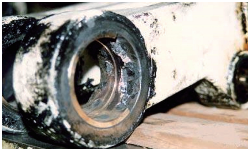
Toggle Link Bushing with Advanced wear (Mould Clamping Unit)
