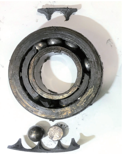
Damaged Bearings due to Lack of Lubrication
